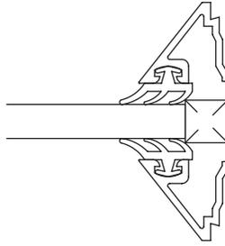
1/4" GLAZING WITH EXTERIOR AND INTERIOR GRID
